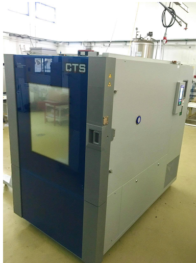
FIGURE 4 – The climatic chamber used in tests
