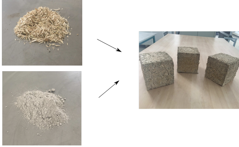
FIGURE 3 – Formulation of the 15 \times 15 \times 15 \text{ cm}^3 samples
