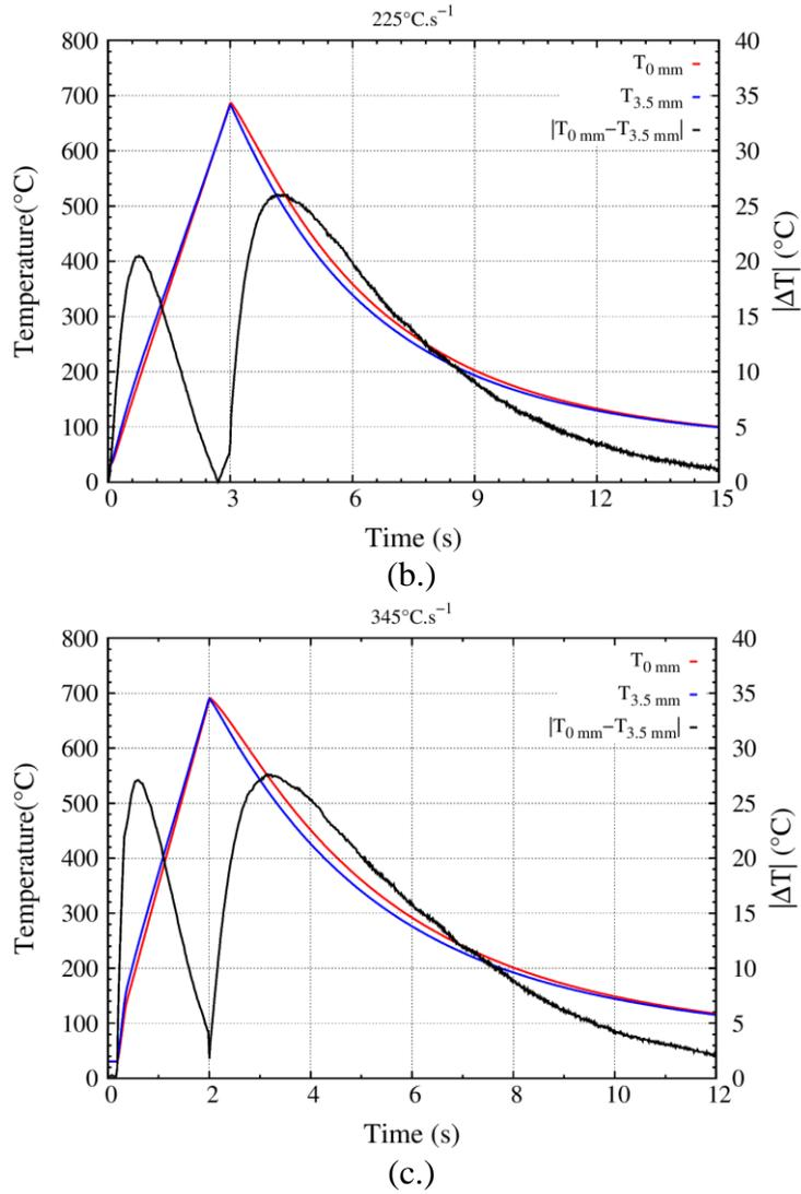
Figure 3. Temperature difference at (a.) 28, (b.) 225 and (c.)  $345 \text{ }^\circ\text{C} \cdot \text{s}^{-1}$
