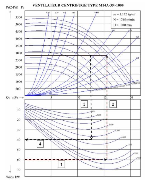
Figure 7. Chart of the fan FEVI, ref: M14A-3N-1000, barometric pressure = 101325 Pa. Maxi speed = 1850 tr/min, aeraulic performances according to standard ISO 5801
