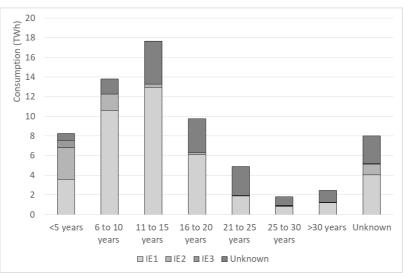
Figure 2. Motors consumption by age and by standard. Source: CEREN 2017 redesigned EDF.
