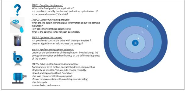
Fig 5. Main steps description for the system approach
