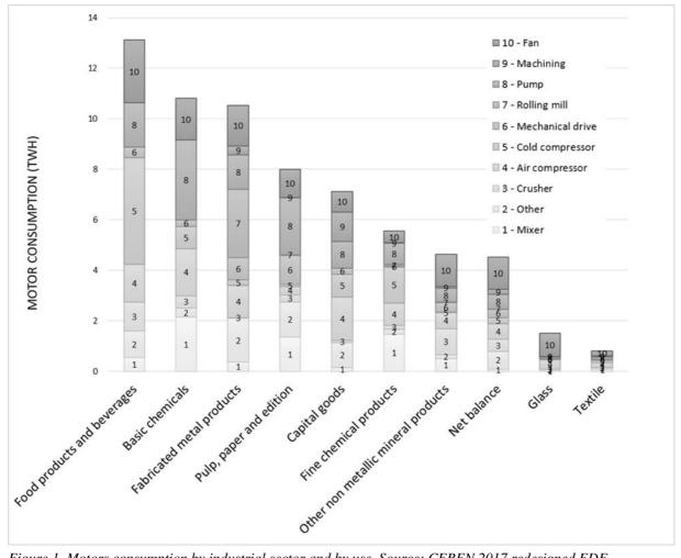
Figure 1. Motors consumption by industrial sector and by use. Source: CEREN 2017 redesigned EDF.
