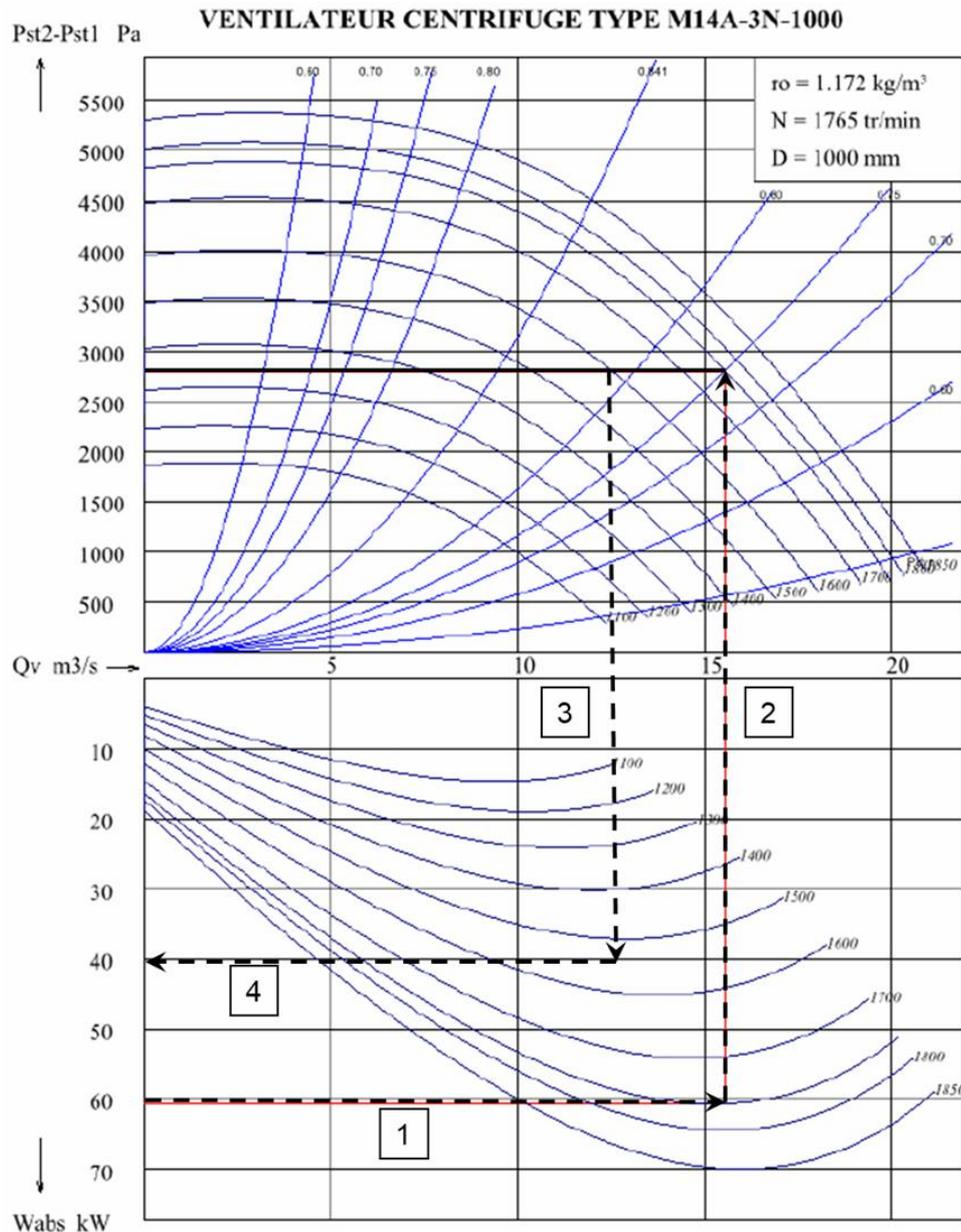
Figure 7. Chart of the fan FEVI, ref: M14A-3N-1000, barometric pressure = 101325 Pa. Maxi speed = 1850 tr/min, aeraulic performances according to standard ISO 5801
