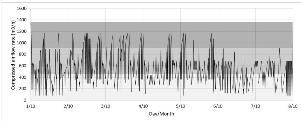
Fig8. Initial load curve of the compressed air flow rate over a week production
