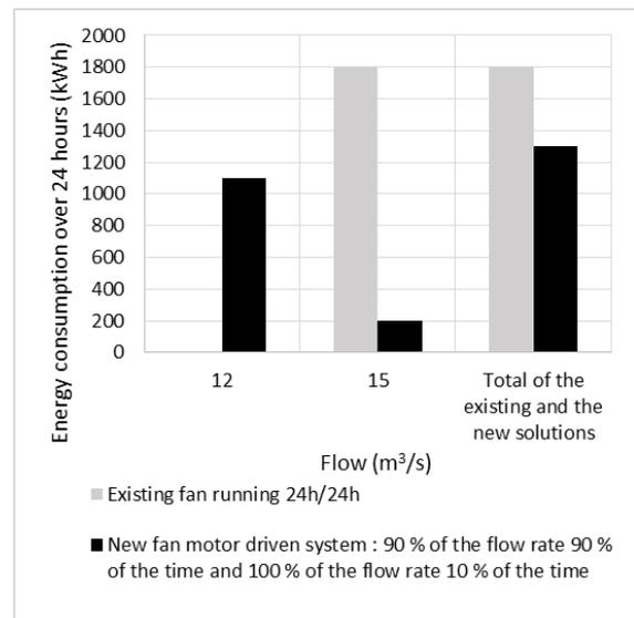
Figure 6. Load curve of the fan from network analyzer Fluke and ESA simulations results
